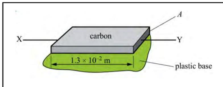
The **resistance** of the carbon layer between X and Y is =  $2200 \Omega$ .
