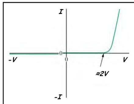
For  $pd (V) < \approx 2V$ , the current ( $I$ ) is  $\approx 0$ , so the LED has almost infinite resistance. The LED starts to conduct at its **threshold  $pd$  ( $\approx 2V$ )** and its resistance decreases dramatically for  $pd$ 's  $> 2V$ .
