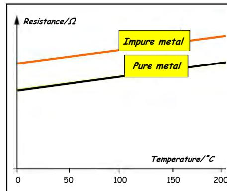
The **RESISTANCE** of an **IMPURE** metal also **increases linearly** with **increasing temperature**, but it is **greater** than that of a **PURE** metal.
